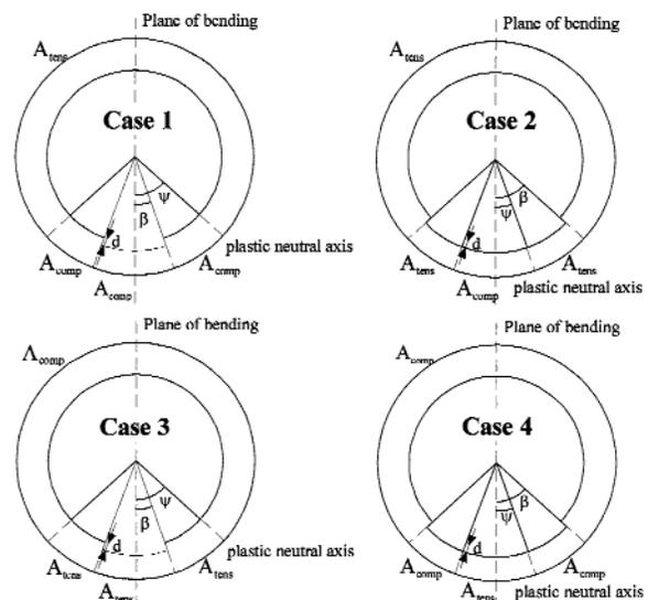
Fig. 1 The 4 combinations of defect and bending
