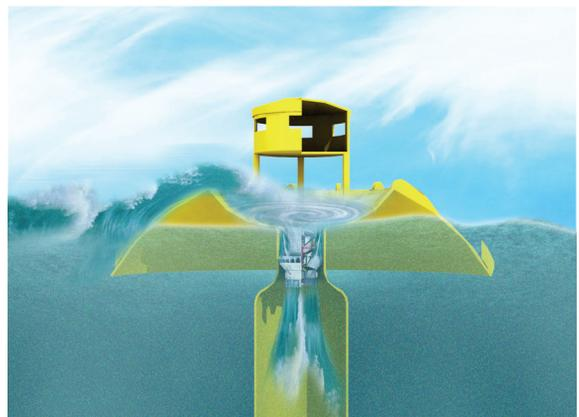
Fig.1 Spiral-reef overtopping wave energy converter
