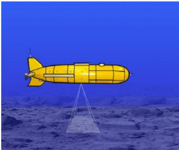
Fig.1. Shooting of the bottom using UUV digital photo system.
