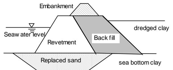
Figure 1 Outline of construction of additional embankment
