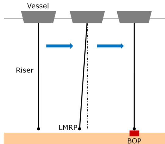
Figure 1 Reentry Control of Riser Hanged Off
