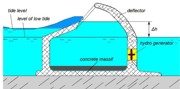
Fig. 1. Simple type of OWEC with low-pressure hydro turbines
