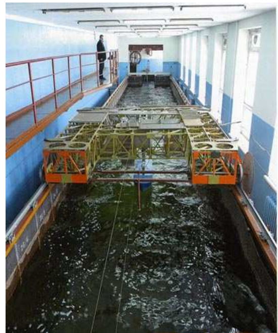
Fig. 1. Testing tank in KnASTU.
