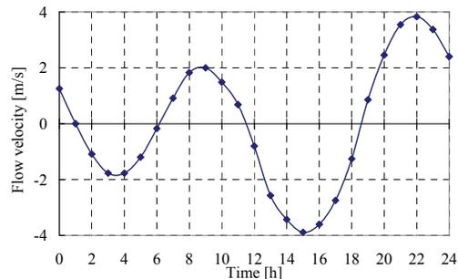
Fig.1 Current velocity curve in Kanmon Strait
