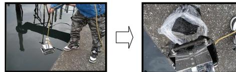
Fig.3 Catching Sludge
