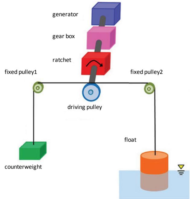
Fig. 1 Schematic diagram of the energy converter
