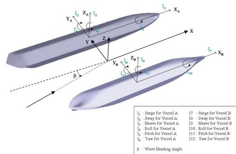
Fig. 1 Coordinate system of two-body motion analysis
