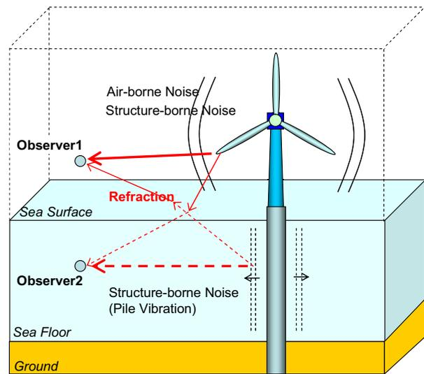
Fig. 1 Noise radiation characteristics in offshore wind turbine
