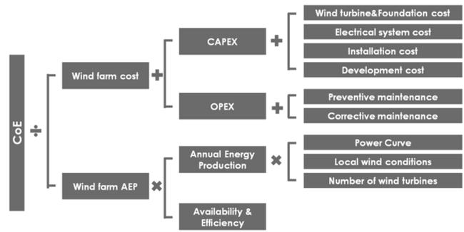
Fig. 2 Modular structure of the tool developed in the OWFLO project (Elkinton et al., 2005)
