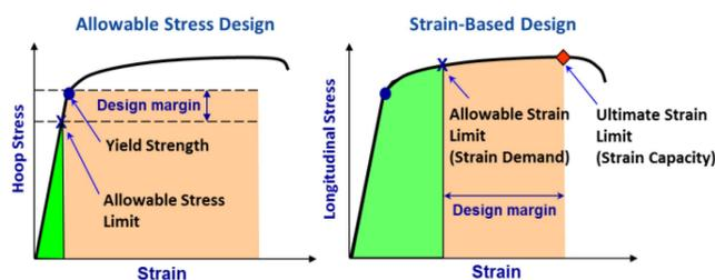
Fig. 1 Principles of SBD versus stress-based design
