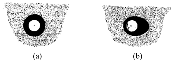
Fig. 1 Idealized normal stress distribution: (a) over pipe at rest, and (b) after a horizontal rightward pipe displacement (after Audibert and Nyman, 1977)
