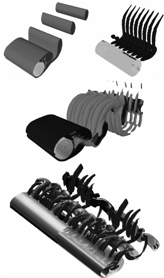
Fig. 1 Dynamics of cylinder wake in 3-D at  $Re = 300$ : 2-D wake (top left), first signature of instability (top right), resultant 3-D wake before saturation (middle), and post-transient established 3-D flow with fully developed hydrodynamic instabilities (bottom, from Poncet, 2004)
