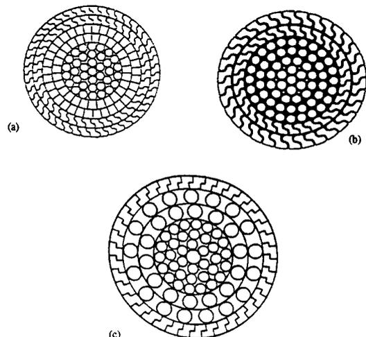
Fig. 1 Typical examples of lock coil cable constructions
